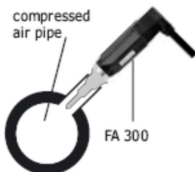
Screw in probe with G 1/2" thread pressure-tight in the center or at the top of the compressed air pipe. Take care that measurement is effected close to the compressed air flow. U-bend pipes or non-flowing compressed air result in very slow reaction times for the moisture reading.
