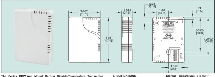
The Series CDW Wall Mount Carbon Dioxide/Temperature Transmitter combines accurate CO2 measurements with a passive temperature output. The Non-Dispersive Infrared (NDIR) sensor continuously updates the calibration through a proprietary logic feature which limits the amount of error due to drift. The CDW series is ideal for building automation systems to help control the fresh air intake in a room.
