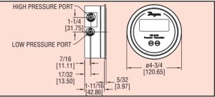
The Dwyer Series DM-2000 Differential Pressure Transmitter senses the pressure of air and compatible gases and sends a standard 4-20 mA output signal. The DM-2000 housing is specifically designed to mount in the same diameter cutout as a standard Magnehelic® gage. A wide range of models are available factory calibrated to specific ranges.
