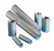
Parker stainless steel sintered metal filters may be used in liquid or gas service, to filter particulate sized from 5 micron to 100 micron - depending on the grade of the filter used. The Parker stainless steel sintered metal filter has excellent chemical resistance characteristics.
