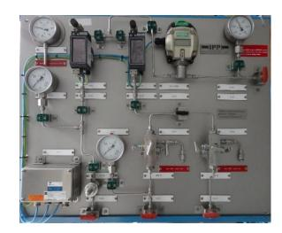
IPP designed, built and tested 16 Gas analysis system panels, according to ATEX and IECEx regulations.
