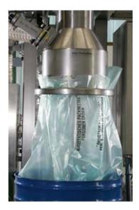
The pressure, which is needed for shaping of the container, must be adapted to the thickness of the interior bag. If the pressure is too small it will not be enough for an ideal shaping and if the pressure is too high it can destroy the container.
