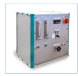
Quality verification of aerospace air ducts by measurement of the leak and flow capacity.
