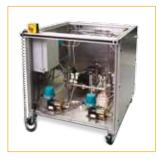
Test stand allows hydrostatic durability and leak test up to 60,000 psi [4000 bar].
