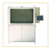
Test stand is for pressure testing of a variety of aero engine tubes over a wide pressure range. Ensures safe operation during testing and provides user with reliable results which can be stored in database for future reference.
