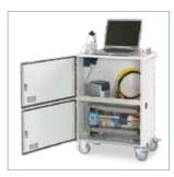
Mobile test rig monitor medical systems in hospitals. Pressure, flow capacity and leakage demands are verified.
